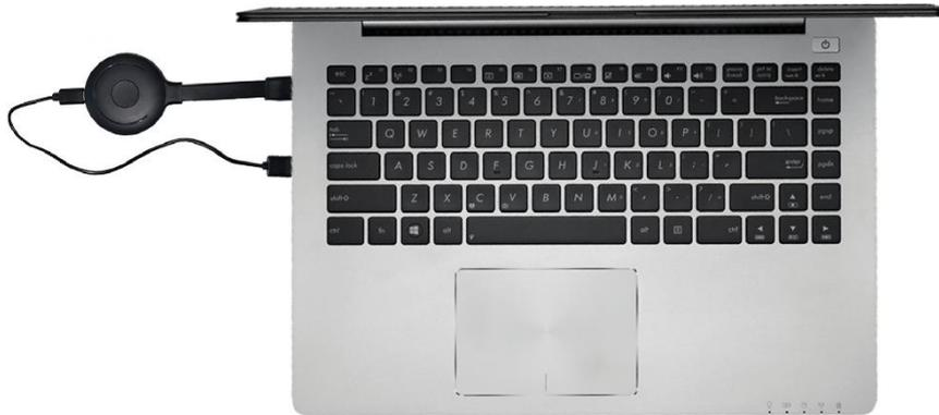
The USB cable must be connected as well as the HDMI cable to provide power to the PushShare dongle if the HDMI port does not provide enough power.
