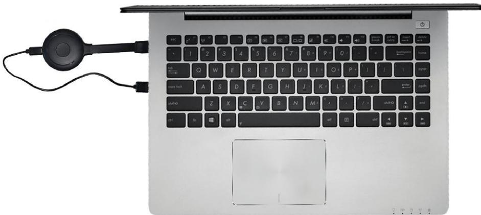
The USB cable must be connected as well, as the HDMI cable will only provide the video and audio signal. The USB will provide the touch functionality.
