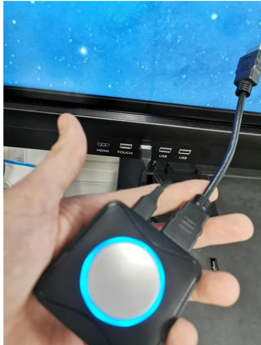
4. Once the pairing is in process, the device will begin to flash.
