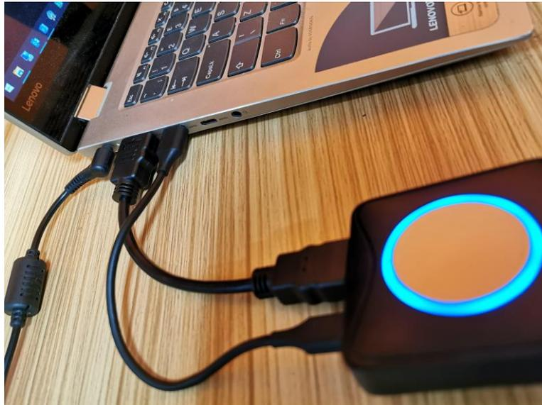
The USB cable must be connected as well as the HDMI cable to provide power to the PushShare dongle.
