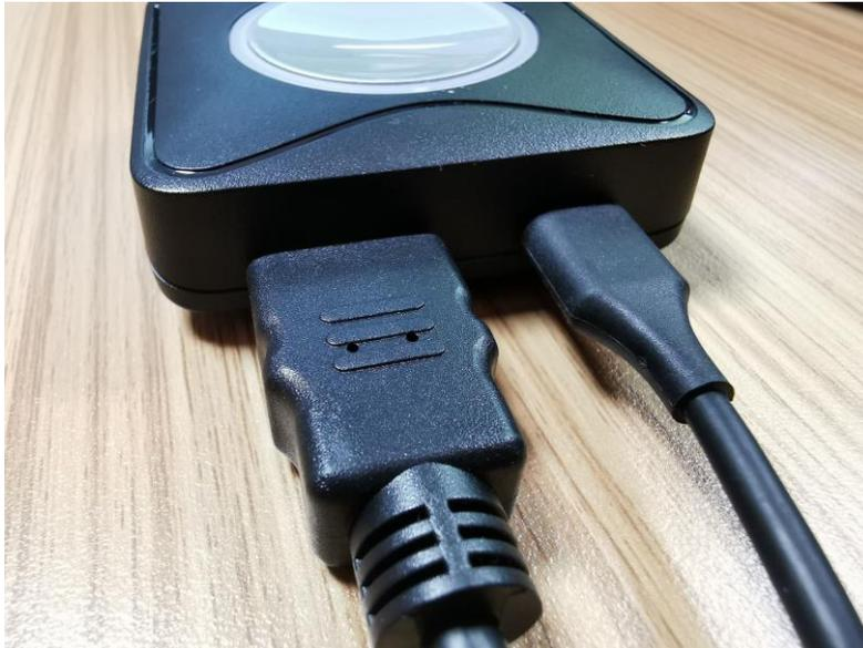
2. Insert the USB and HDMI into the PC you wish to project to the screen.
