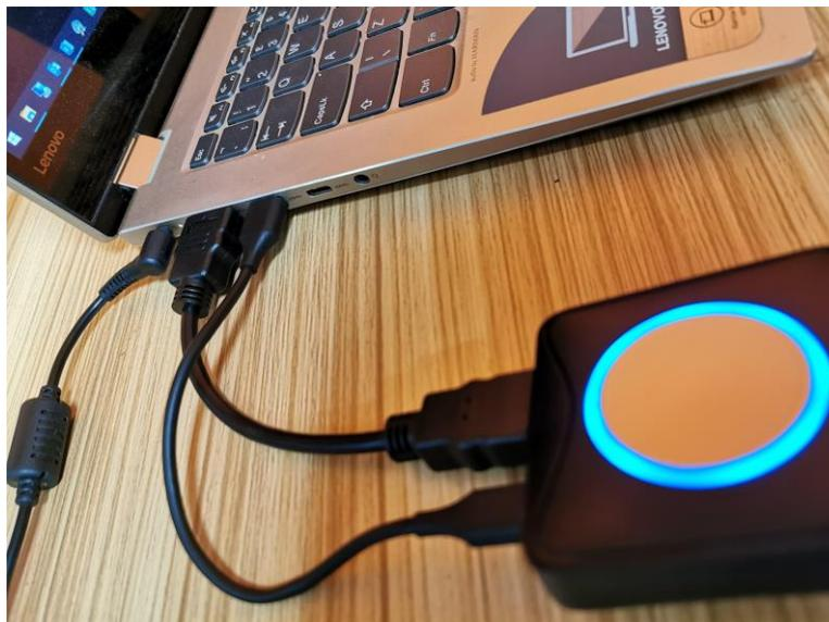
3. Press the button on the PushShare device to activate the device and begin projecting onto the screen.
