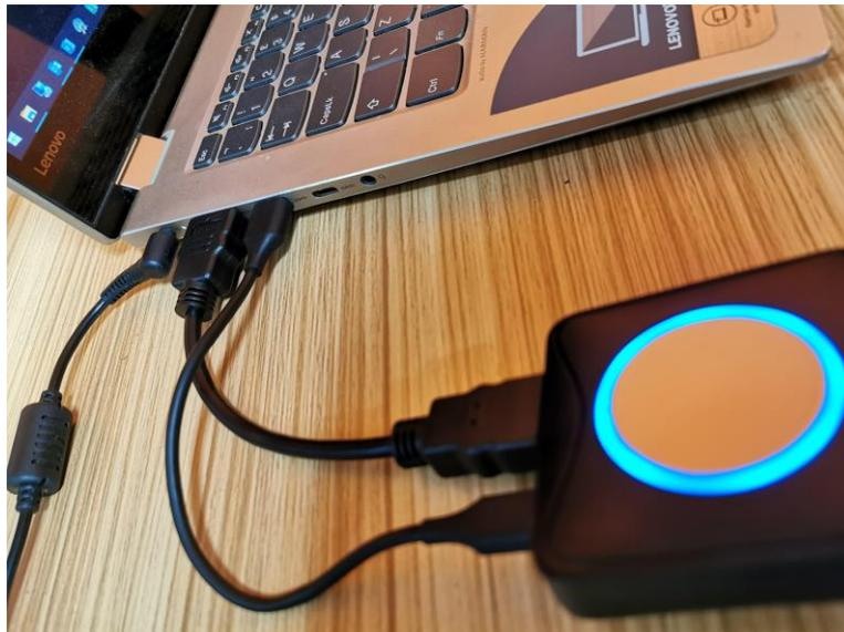
The HDMI cable must be connected as well as the USB cable to send the video and audio signals.
