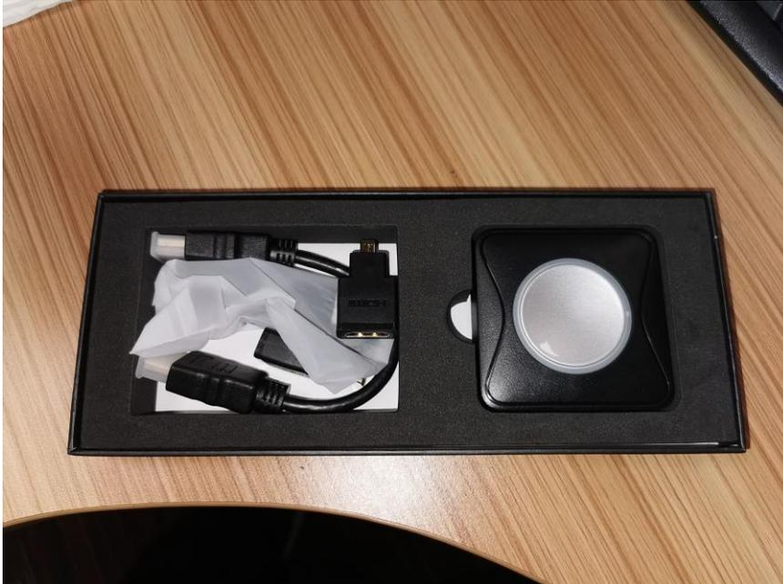
2. Attach the USB and HDMI cable provided in the box to the PushShare device.
