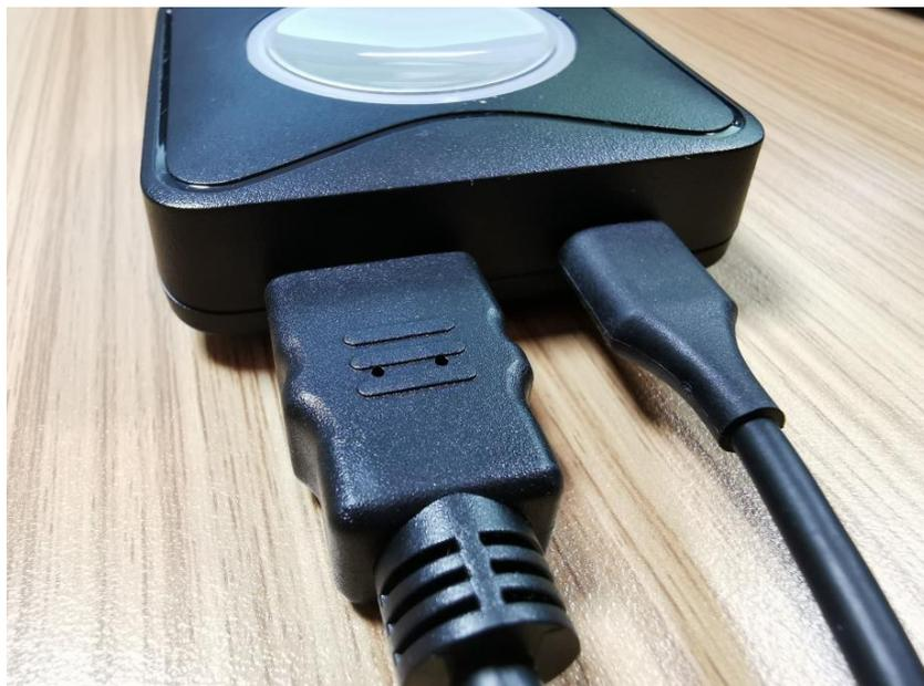
3. Plug the USB cable from the PushShare device to the screen's "USB" input. This will automatically pair with the screen.
