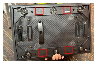
When attaching the LED Module to the cabinet make sure you attach it the correct way up. There are 4 markings on the back of each module with an arrow facing up to show which way it should be installed.
