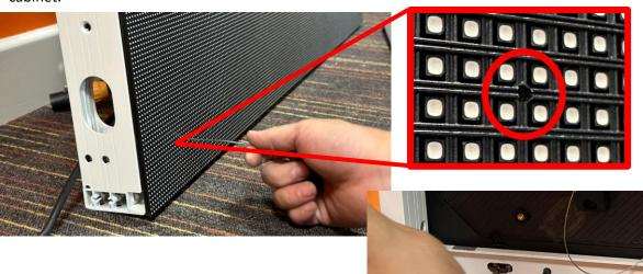
You can also remove the modules from the back. Simply twist the 4 clips to detach the module from the cabinet.
