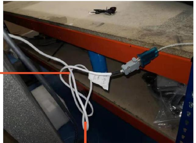
The RS232 Cable provided to be able to connect to the computer; multimedia software will be inserted into the 'RS232 in' Slot
