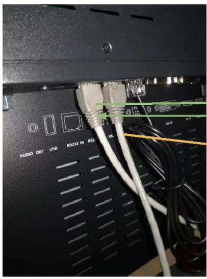
The RS232 cable is then connected to the second screen in the 'RS232 in' input.
