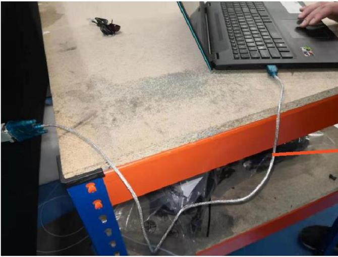
Use the cable provided (VGA to USB) to connect to the RS232 cable will need to be inserted into an empty USB slot, exactly like the picture shows.
