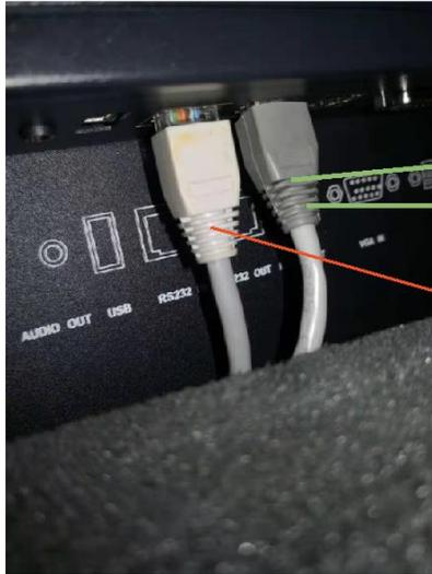
This RS232 cable is connected into the 'RS232 OUT' input, and this cable will be connected to the second screen shown on the image below.
