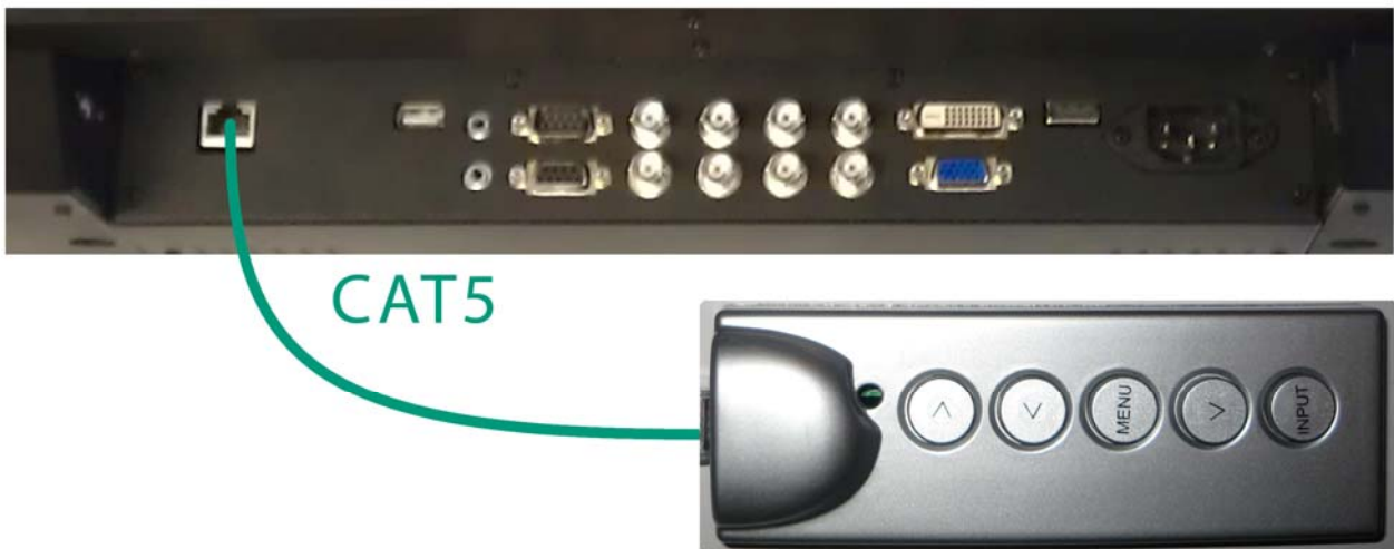
Figure 6 Serial Control Box to Screen Connection
