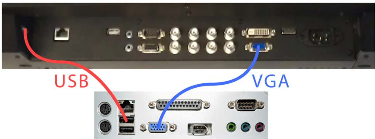
Figure 5 Screen to PC Connections
