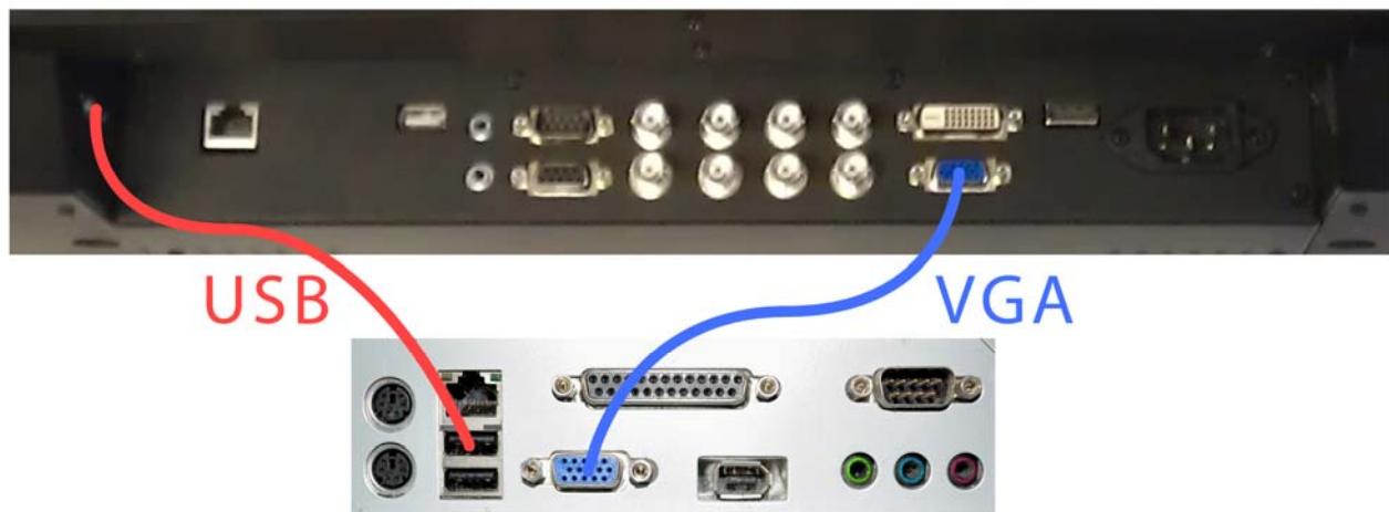
Figure 1 Screen to PC Connections
