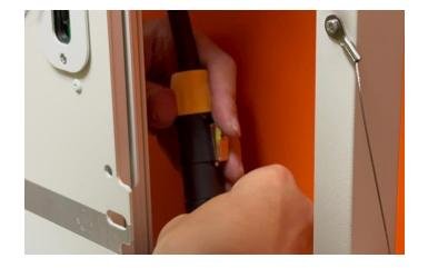
**Step 7**Once all cables have been attached, you now need to re attach all the LED modules to the cabinet.
